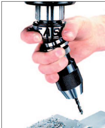
3. Removing drill chuck holder with one hand.
