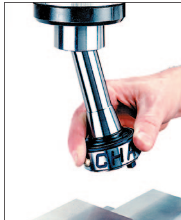
1. Loading the Quick-Change Body into a standard R8 spindle.
