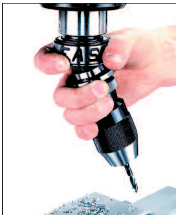
3. Removing drill chuck holder with one hand.
