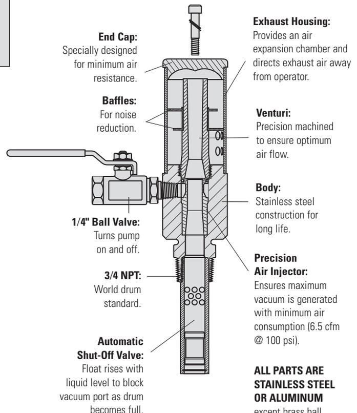
**ALL PARTS ARE STAINLESS STEEL OR ALUMINUM** except brass ball valve, Delrin float and Buna-N O-ring.
