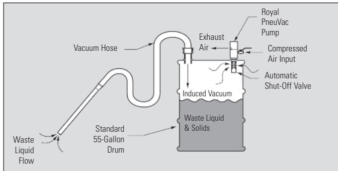
**Heavy Duty Construction** – Entire pump (except ball valve, float and O-ring) is made from either stainless steel or aluminum. Other brands are made from rust-prone carbon steels and light-duty plastics.
