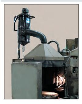
Grinding applications can sometimes be more demanding than typical turning and milling applications because grinding produces fine dust particles that become entrained in the mist stream. Over time, this dust can accumulate on the drum pads, resulting in the need for more frequent maintenance. If regular maintenance is not performed and a significant volume of solid matter builds up in the drum, balance and vibration issues may arise.
