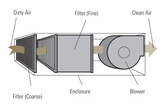
**High Operating Costs** The biggest drawback of media-type filtration systems is the high operating cost associated with replacement filters. These filters are designed to retain contaminants, so they will become clogged with use. Usually they are made from media that cannot be cleaned, so the only alternative is replacement. Depending upon the cost of the filters and the replacement frequency, this type of system can be quite expensive to operate over the long term.
